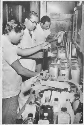
A STEADY stream of "cuts" moves from the "TB" stills to this workbench where Ramon Croes (left) is shown taking their A.P.I. gravity. B. F. Dirksz (center) is recording the various cuts taken while J. A. Richardson is checking their weight.
